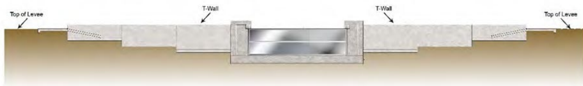
Figure 3: Conceptual Stoplog Gate - Elevation View with Gate in Open Position (Crane not shown for clarity)
