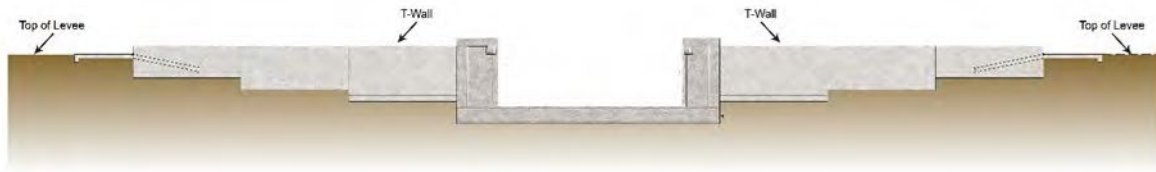
Figure 3: Conceptual Stoplog Gate - Elevation View with Gate in Open Position (Crane not shown for clarity)
