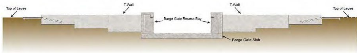
Figure 3: Conceptual Barge Gate - Elevation View with Gate in Open Position
